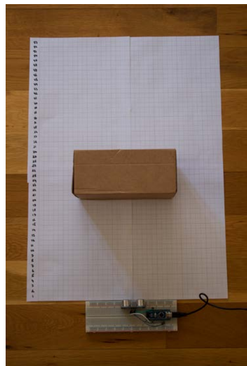
Figure 19. HC-SR04 Ultrasonic Distance Sensor Accuracy Test Against a Fixed Obstacle
